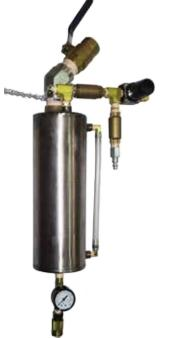
The tool drastically reduces service time and maintenence costs as it does not require the removal of the DPF. This helps to extend the life of the DPF, improve the performance of the filter and reduce untimely regenerations thereby increasing uptime.
